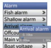
In order to obtain a more precise positioning from the target point, you can set it to a smaller value, for example: 2 meters or even 1 meter.
