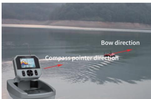
Note: For electronic compass,  $\pm 15$  degrees is the allowable error range. So while the boat is moving, if you find a small deviation between the compass needle direction and the bow direction, this is normal.
